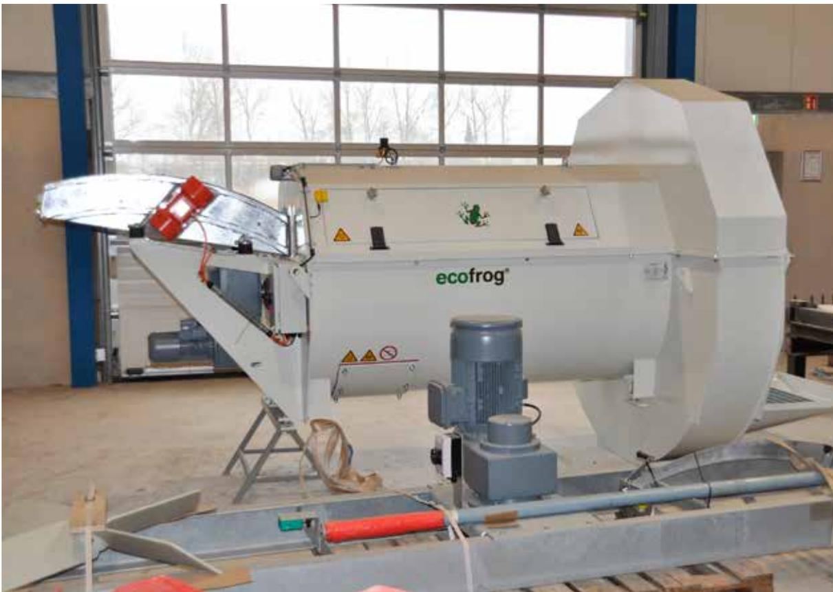
Ecofrog GmbH supplied an RE\_X04Z residual concrete reclaimer with feeding wheel
