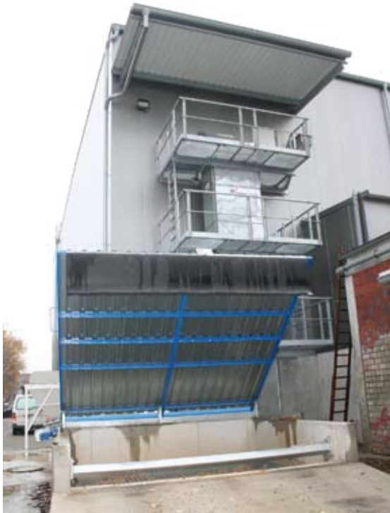
Fig. 4 The truck discharge bunker with ground level access feeding the double belt conveyor by means of a discharge conveyor.
