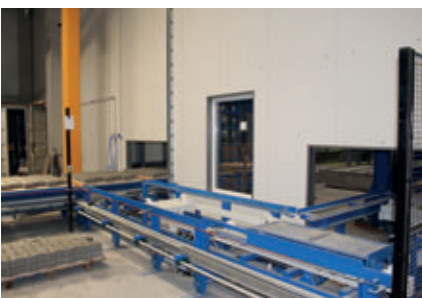
The production boards from the two lowerators are merged via a bypass onto a common transport line, a slideway.
