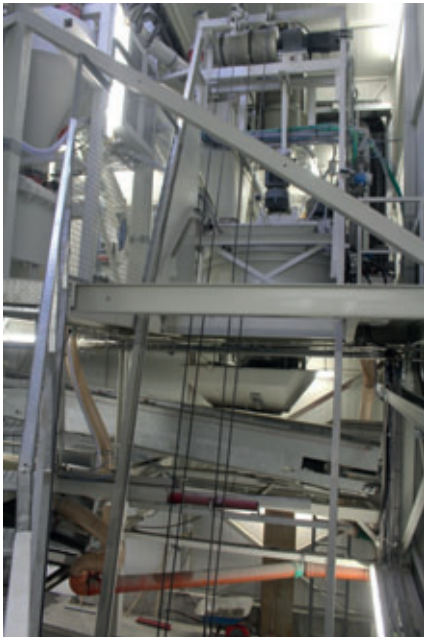
Facing concrete mixer from Kniele; it empties onto a conveyor belt below the mixer
