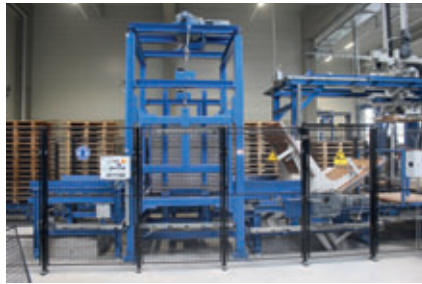
The boards are automatically brushed, turned by the board turner and automatically collected and stacked by the board stacking device.
