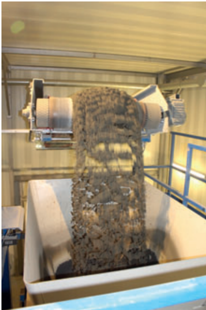
The concrete mixers empty onto discharge belts that transport the concrete into the silos of the block making machine.
