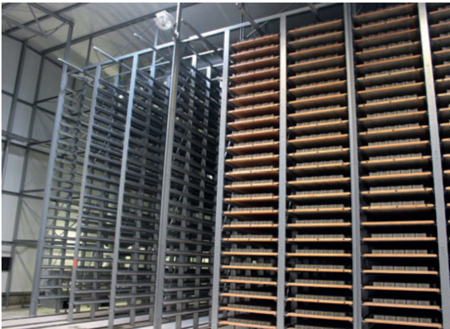
Specially galvanised curing rack from HS Anlagentechnik for 4186 production boards
