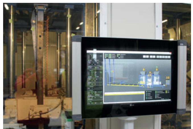
Windows in the noise insulation enclosure allow a very good view of the Frima HP1200 while the production can be followed in real-time on the monitor.
