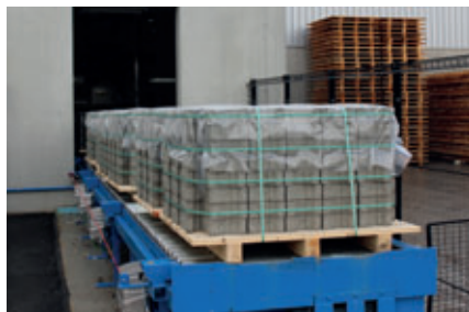
The fully packaged stone packets stand on the buffer conveyor awaiting removal by the fork-lift truck
