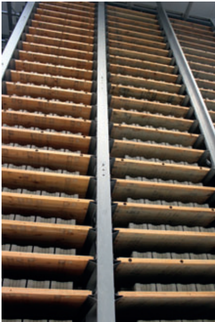
A special feature from HS Anlagentechnik is the special support profile with a length of up to 9 m
