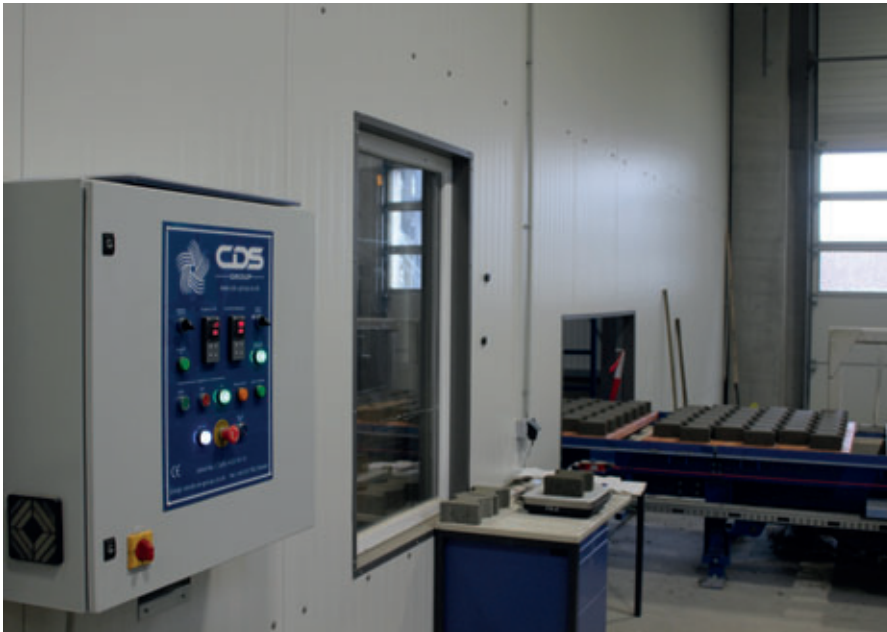
The fresh products are transported by a walking beam conveyor on the wet side to the elevator with 23 levels
