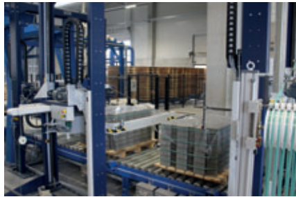
The finished stone packets move via a roller conveyor to the cover sheet feeder and the strapping machine from Cyklop.
