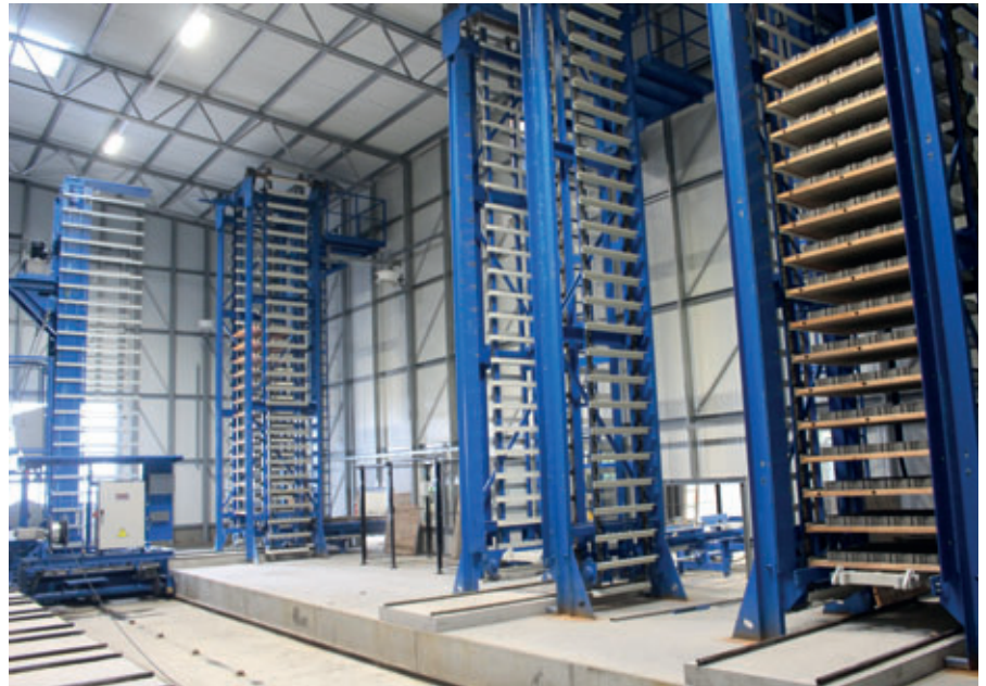
The dry side is served from the drying chamber by two lowerators.
