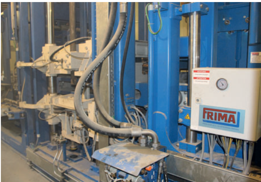
The HP1200 can be used for the production of numerous concrete building materials such as pavers, kerbstones, concrete slabs, hollow masonry blocks or garden elements.
