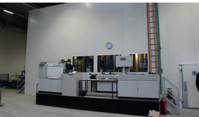
Central control station for all system components in front of the CDS noise insulation enclosure for the Frima block making machine
