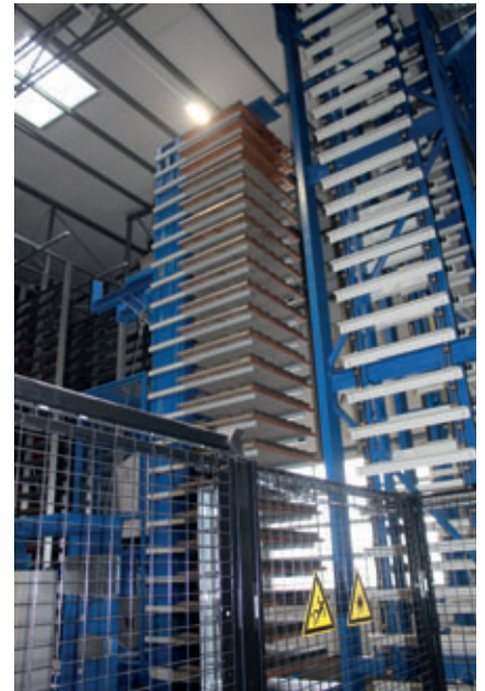
Once the elevator is completely filled, the Frima finger car takes over the fresh products on the 23 production boards.
