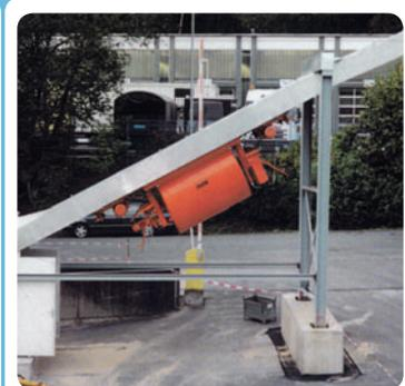
Rollover bucket in a 32° inclination = 60%
