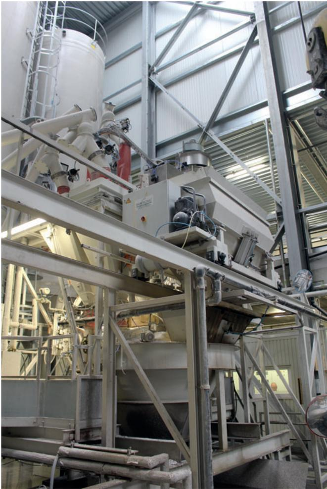
*The aggregates are transported directly to the mixer and the mobile scale is emptied into it.*
